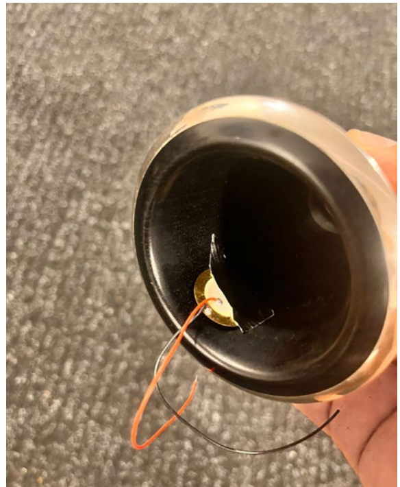
Figure 1. A Piezo Vibration Sensor placed inside the clarinet's bell.
